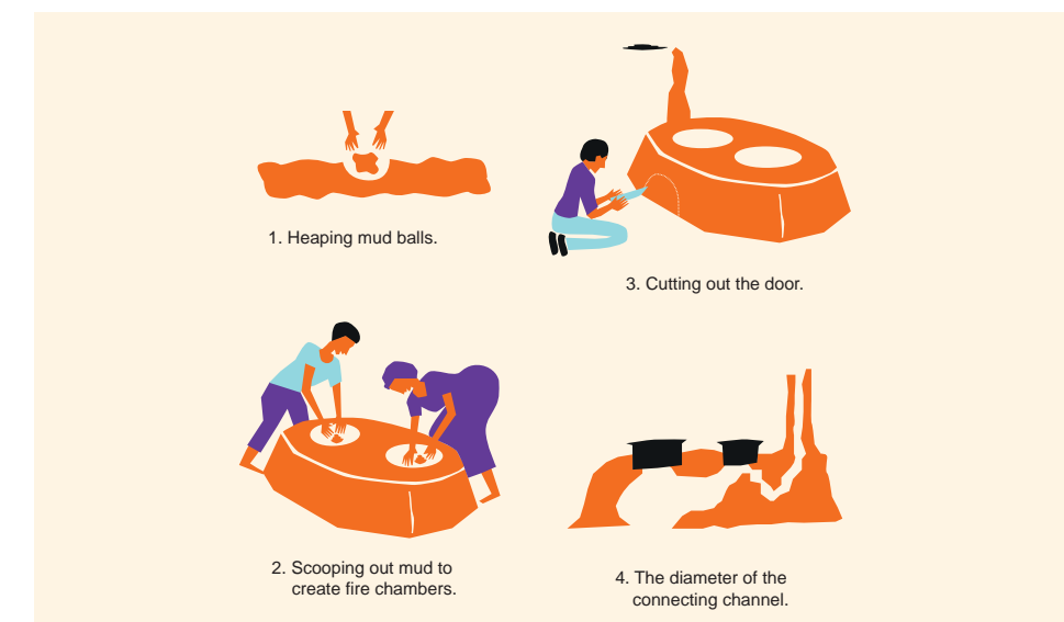
Illustration: How to build a wood saving stove
